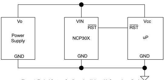
Figure 2. Typical System Configuration Using with Supervisory Device $\checkmark$
